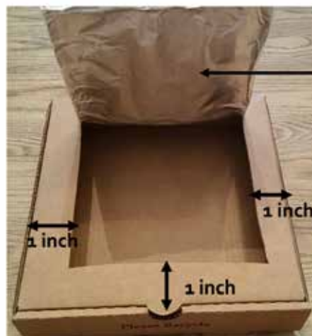
Figure 2: Creating a reflector to reflect sunlight inside the solar oven (box).
