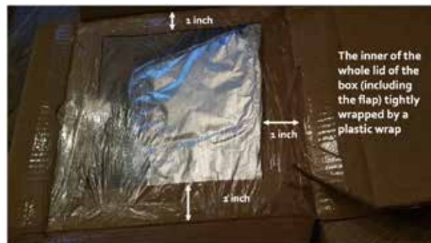
Figure 3: Creating an airtight window to keep more heat inside the solar oven (box)
