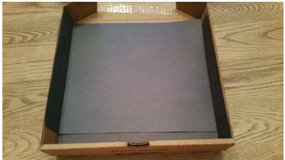
Figure 4: Making the oven more energy efficient by adding a dark surface to absorb more energy.
